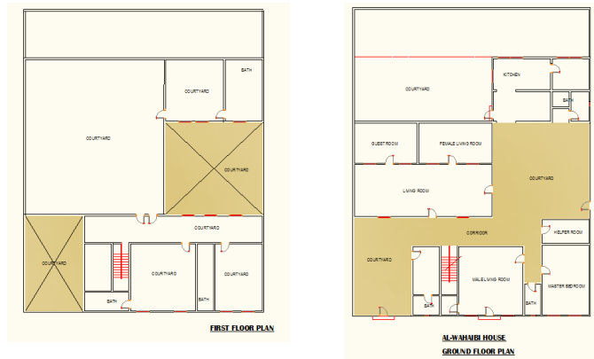
Fig. 10: Plan of coastal courtyard house at Quriyyat (source: author)
